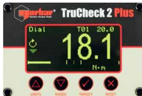
TruCheck™ 2 Plus display showing below target tolerance
