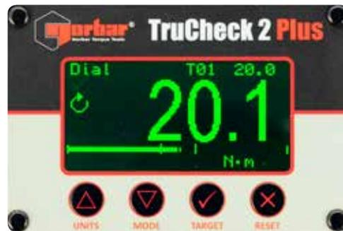
TruCheck™ 2 Plus display showing within target tolerance
