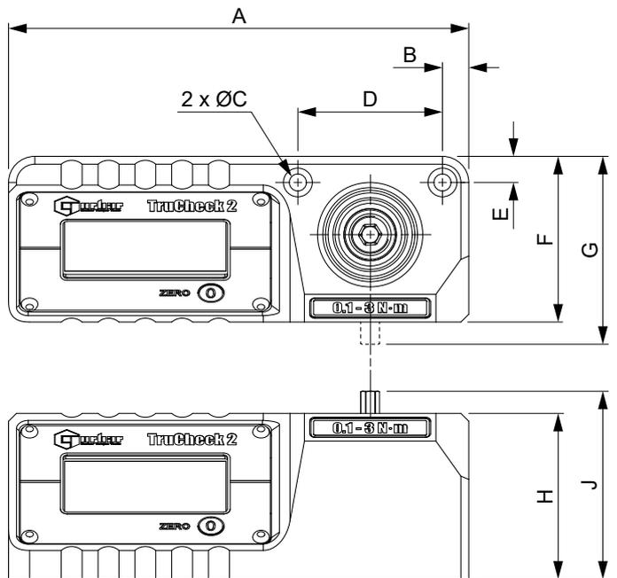
NOTE: The male hexagon on the 3 N·m and 10 N·m models is vertically aligned. The 30 N·m model male hexagon is horizontally aligned.
