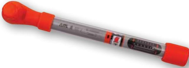
Using injection moulded Nylon 11, Norbar's insulated torque wrench complies with IEC 60900:2004 and is more durable than the traditional PVC dipped insulated tools. Certified to 1,000 volts.
