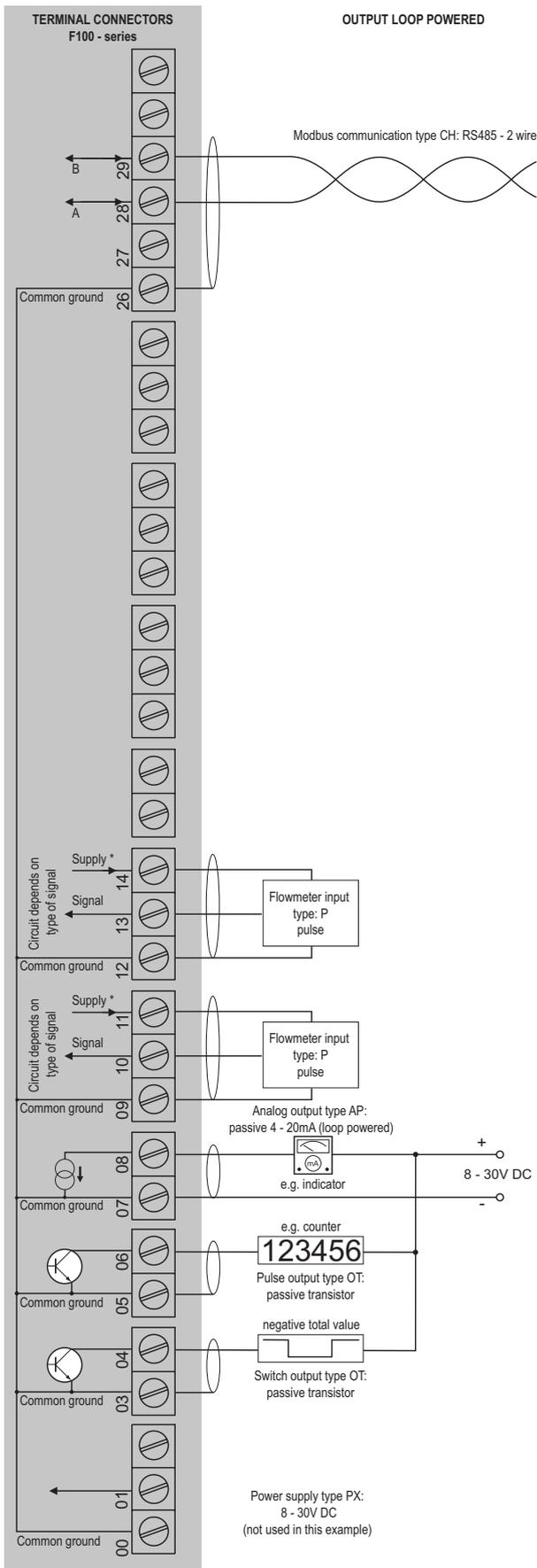
\* For pulse type inputs:  $V_{ref}$ : 1.2V/3.0V available.- NO power output, available  $I_{supply}$ : <1mA. Note: using these ref. voltages at max. load, will reduce battery life significantly.
