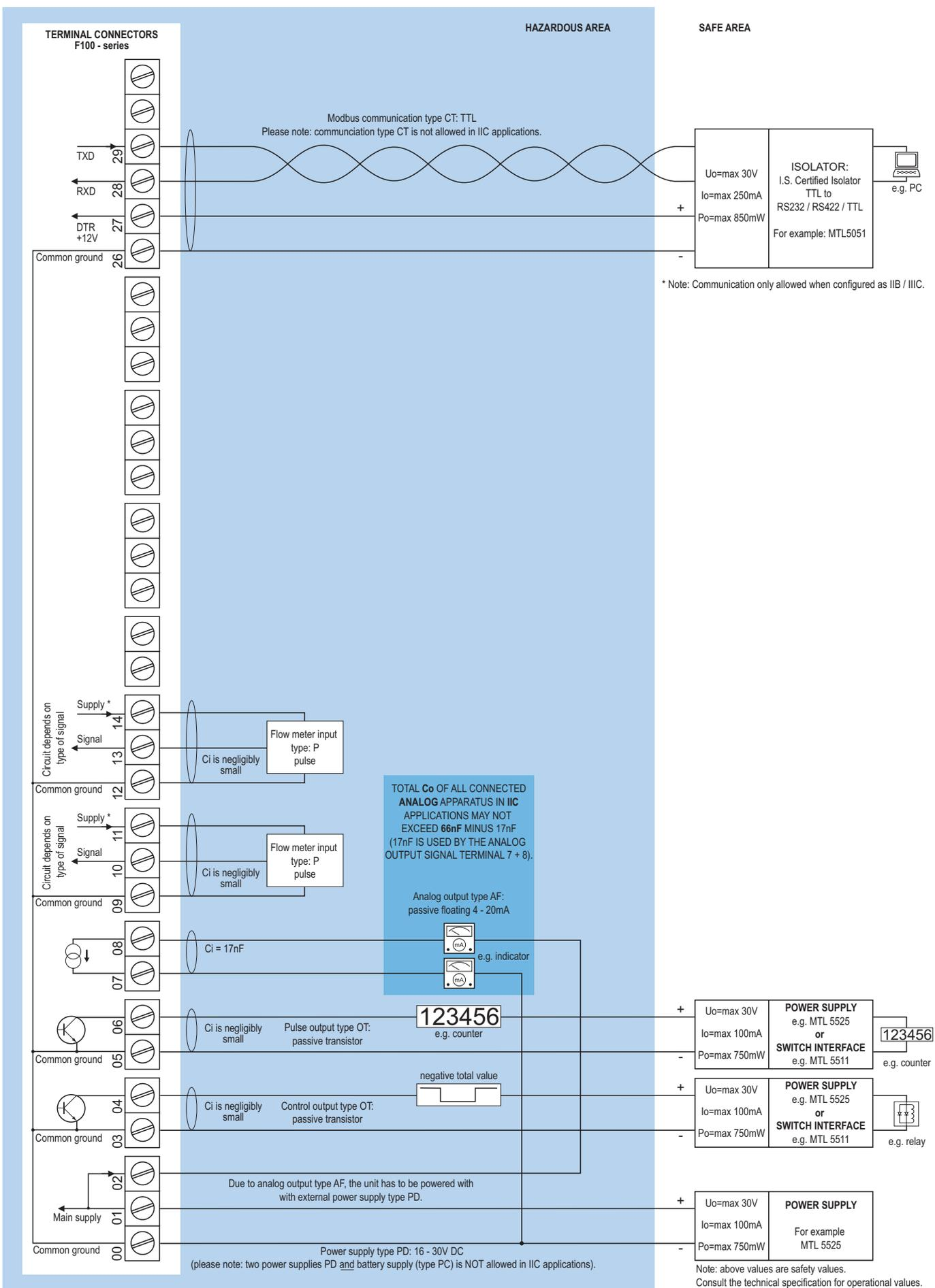
\* Note power supply type PD: the supply voltage to pulse sensors is maximum 8.7V (Uo=max 8.7V Io=max 25mA Po=max 150mW) and to analog sensors as connected to terminal 1 (internally linked).
