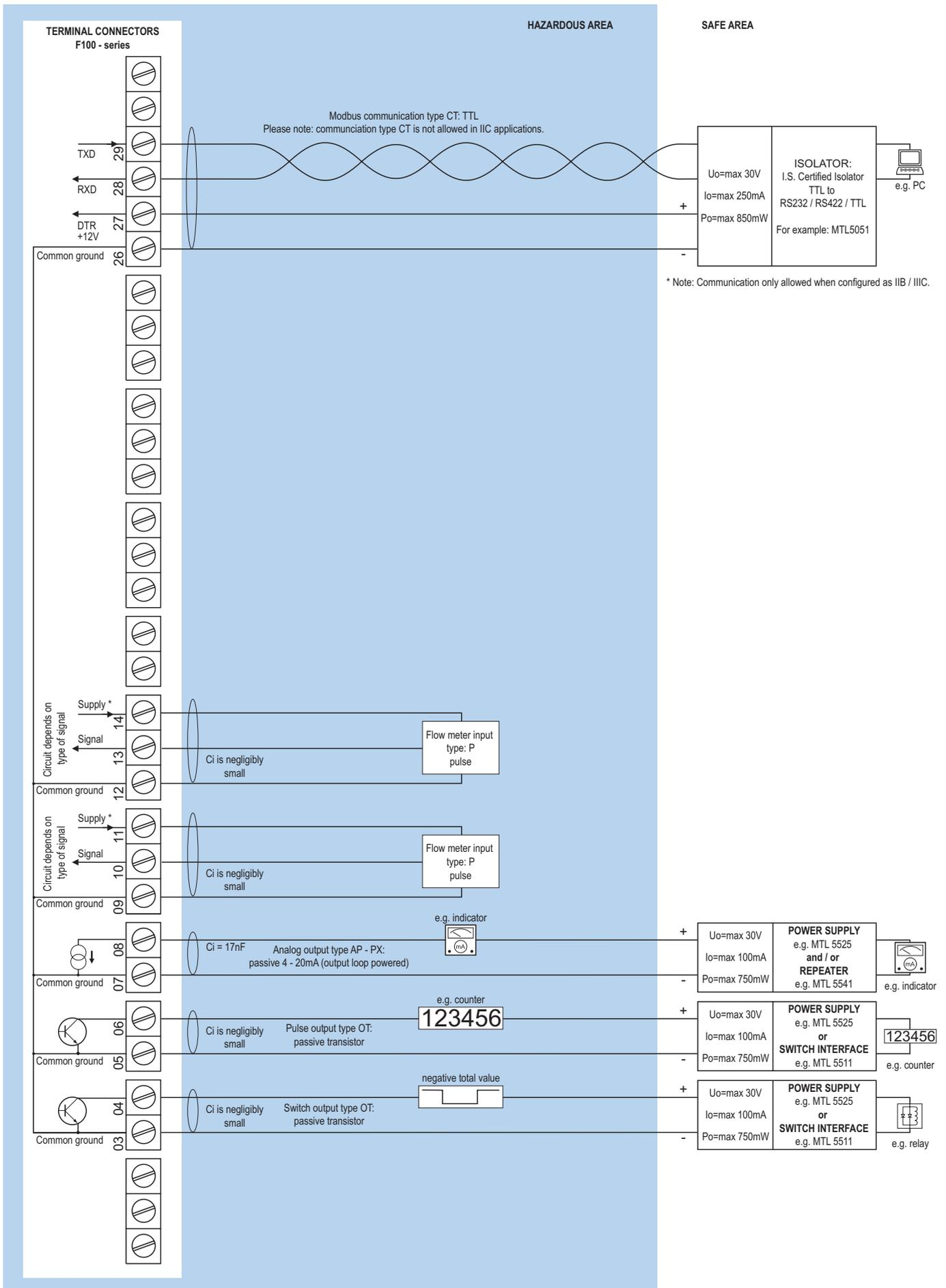
\* For pulse type inputs:  $V_{ref}$ : 1.2V/3.0V available.- NO power output, available I<sub>supply</sub>: <1mA.
