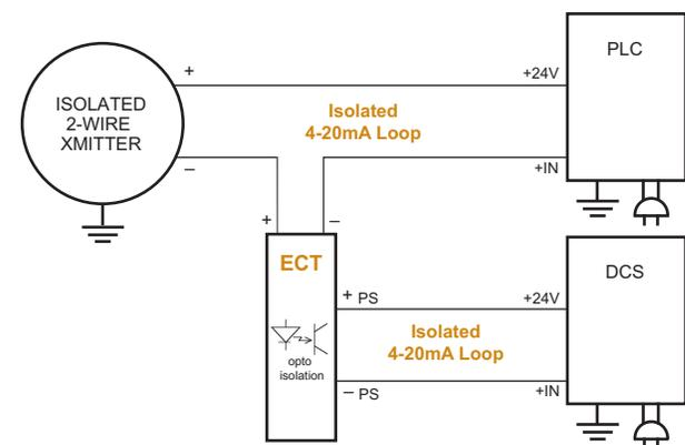
Figure 3. Boost process signals to allow another instrument to be added to an otherwise overloaded loop.
