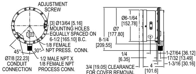
The **Series PG Gas Pressure/Differential Pressure Switch** has a large sensitive diaphragm and a reliable time proven mechanical design. For use with air and other compatible gases, they feature excellent  $\pm 1\%$  of full-scale repeatability, clear easy-to-read scale and convenient external set point adjustment.
