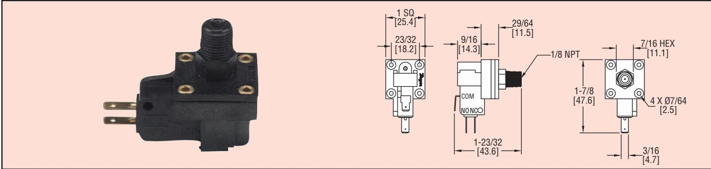
The Series MHS Miniature High Sensitivity Pressure Switch offers a wide range of field adjustable pressure set point options. The compact switch can be used with air or other compatible fluids. Ideal application is for turning pumps and compressors on and off when levels change. The Series MHS models offer a variety of electrical ratings to suit application needs. The switch is easy to install and easy to adjust, with a long mechanical life of over 10 million cycles.
