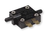
The **Series MDS Miniature Pressure Switch** is designed with a double diaphragm to protect false actuation due to shock and vibration. This low cost pressure switch has a minimum 20 million cycle life expectancy, and an extremely fast response time, making this an ideal device for OEM orders.
