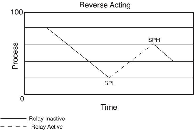
The following alarm function SUB MENUS are activated when  $\square + rL$  is set to SPRL :
