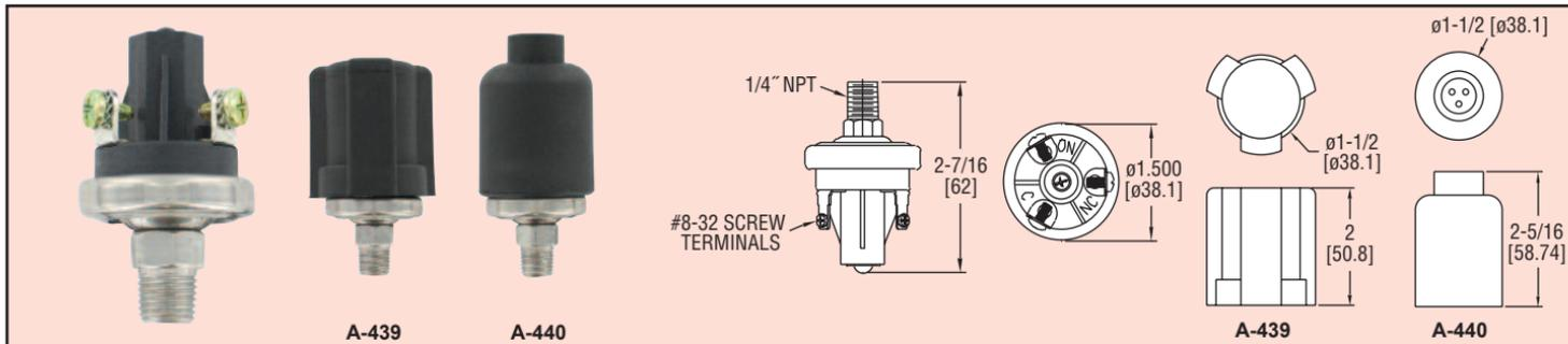
**Series A6 Durable Pressure Switches** have been specifically designed to stand up to extended duty applications. These switches are constructed with a polyamide film diaphragm and are compatible with a variety of fluids. For ease of installation, the switches come with a 1/4" male NPT process connection and can be mounted in any orientation. The Series A6 pressure switches are compact and have great setpoint integrity, and feature simple, easy set-point field adjustment.
