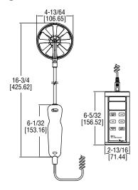
The MODEL 473B 100 mm Vane Thermo-Anemometer Test Instrument is a versatile unit that quickly and easily measures air velocity or volumetric air flow, as well as air temperature and humidity in imperial or metric units. A stainless steel 100 mm vane probe is included, which has a comfortable hand grip and etched insertion depth marks. The extruded aluminum housing fully protects electronics, yet is lightweight and comfortable to hold.
