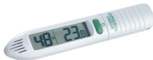
**INSTRUMENT OPERATION** - Insert the battery into the battery compartment located at the end of unit. The instrument will perform a self-test, and within five seconds the ambient readings will be displayed. The unit is switched on/off by pressing the button located on the front. The instrument monitors the humidity and temperature simultaneously.
