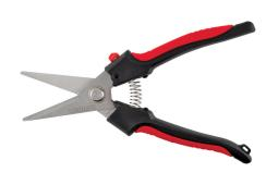
For cutting cardboard, leather, rope, cord, wire, paper & many other materials. Precision ground & hardened stainless steel blades - HRC 50-54 - with one serrated cutting edge to reduce slipping. Lightweight polypropylene handles with spring loaded action. Easy reach safety thumb lock, convenient for right & left hand users. Straight Cutters: Overall length: 203mm (8"), Cutting length: 50mm (2") Offset Cutters: Overall length: 190mm
