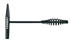
Scaling and chipping hammers. For boiler scaling, weld dressing etc. Spring Steel Shaft Hardened and tempered steel head chisel edge and point striking faces with epoxy coating. Spring steel impact absorbing handle for user comfort.
