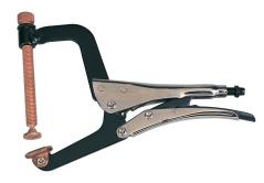
Fine spindle clamping adjustment enables accurate clamping. Swivel joint clamping points allow tapered surfaces to be securely clamped. Copper plated spindle and clamping points ensure weld splatter will not adhere.
