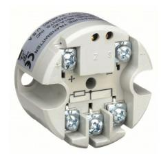
DWYER Temperature Transducer | Range 32 to 392 Degrees F | 10 to 32V DC, | Type K Thermocouple | 4 to 20mA DC | Screw Terminals,
