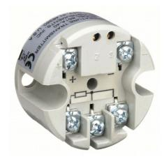
DWYER Temperature Transducer | Range 32 to 752 Degrees F | 10 to 32V DC, 651 | Pt100 RTD, 4 to 20mA DC | Screw Terminals,
