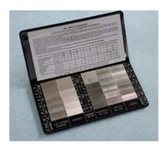
In cases where surface roughness needs to be measured with great precision, elaborate instruments must be used. These are expensive, and often unsuitable for workshop use, where roughness of machined surfaces can usually be assessed conveniently and with sufficient reliability using visual and tactile (fingernail) comparison with a standard set of surfaces machined in the same way.
