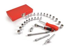
Ideal for assembly and servicing of small precision mechanisms associated with electrical, electronic, ignition and refrigeration work. Sockets have a knurl feature to give a high grip which is essential for a quick tool change when your hands are greasy/oily. Six point bi-hexagon side drive design gives a higher torque than normal sockets, grips worn nuts and will not round off existing nuts.
